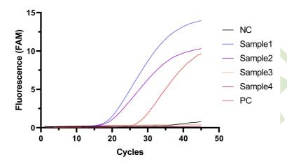
In the figure above, the positive control (PC) shows a CT value less than 35 with a clear amplification curve, while the negative control (NC) exhibits a CT value greater than or equal to 35 with no significant peak.
